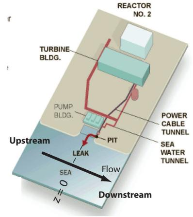
Figure 3: Radioactive water leaked into ocean from the Fukushima power plant
