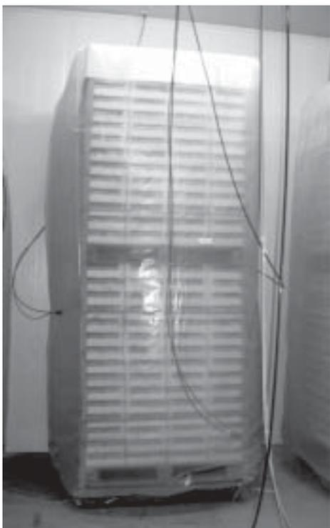
Figure 5. Boxes of red currants in CA storage. Bag is sealed at base of pallet with sensing and gas-feed lines attached.
