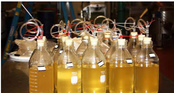
Vessels and test apparatus used to determine elemental sulfur from spray applications in fermenting wines and juice. One goal of the project is to find out how long before harvest sulfur applications need to be stopped to avoid impacts during fermentation.
