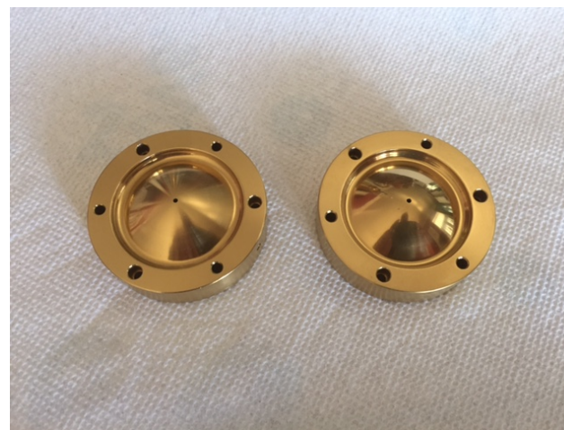
Coating the cathode surfaces with titanium nitride also failed to suppress the discharge.
